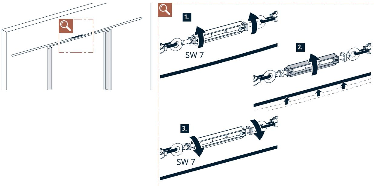
**!** Tighten the lock nuts to prevent loosening!
